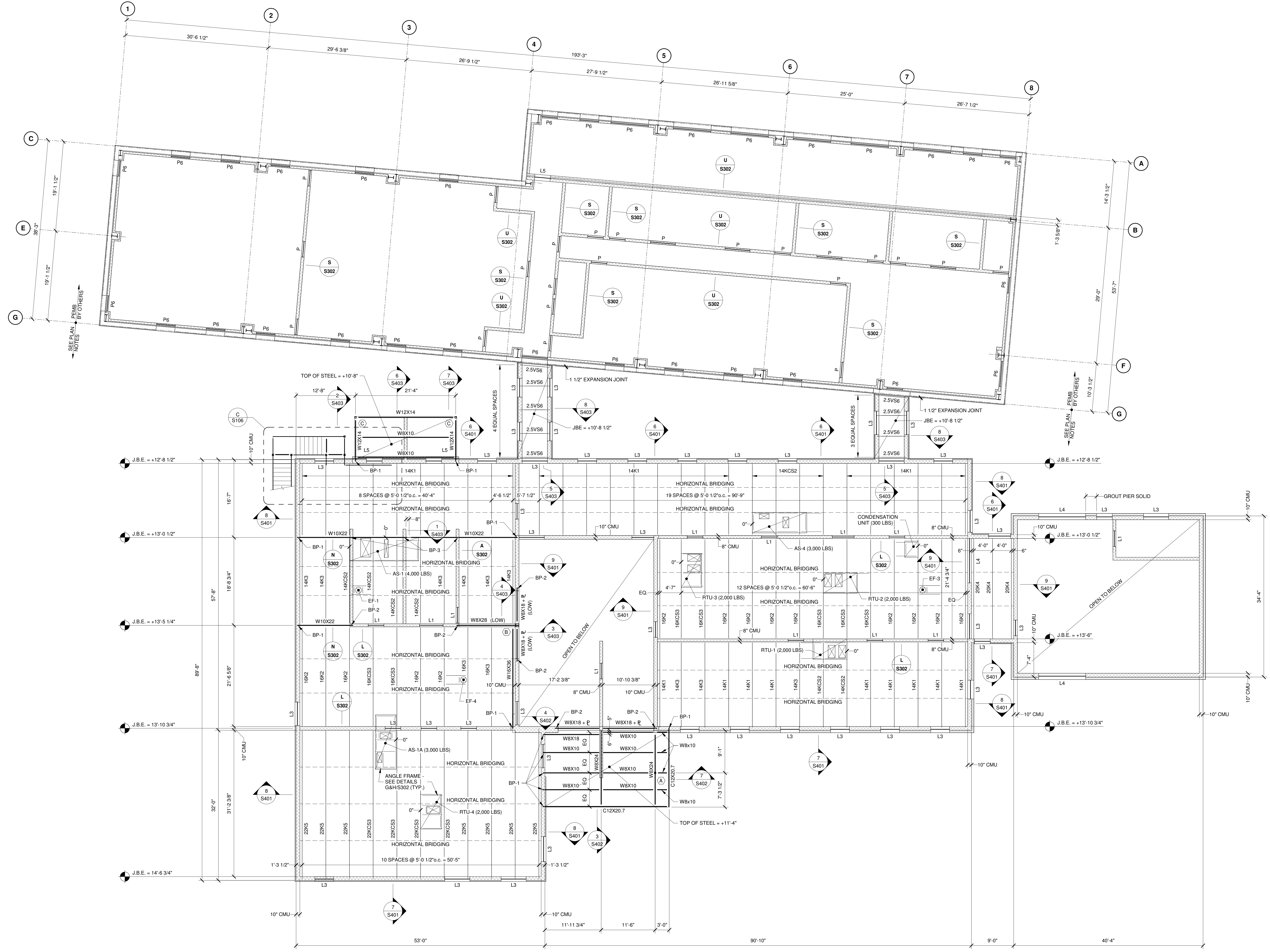
MAIN ROOF FRAMING PLAN 1/8" = 1'-0" NORTH PROJECT NORTH 1. ENTIRE MAIN ROOF DECK TO BE 1 1/2" 22ga. GALVANIZED TYPE 'B' METAL DECK AS MANUFACTURED BY VULCRAFT OR APPROVED EQUIVALENT, UNLESS OTHERWISE NOTED. 2. STEEL JOIST BEARING ELEVATIONS ARE NOTED THUS J.B.E. - 'X'-X" IN PLAN AND ON SECTIONS AS REFERENCED FROM DATUM ELEVATION 0'-0". 3. — IN PLAN REPRESENTS COMPLETE PENETRATION MOMENT CONNECTION. SEE DETAILS AND SECTIONS. 4. DESIGN ALL JOISTS FOR A NET UPLIFT OF 15gpi. PROVIDE ADDITIONAL BRIDGING AS REQUIRED. 5. STEEL BEAMS PARALLEL WITH JOISTS TO BE AT SAME ELEVATION AND SLOPE AS THE JOISTS. 6. ALL DIMENSIONS ARE TO FACE OF CMU WALLS, UNLESS OTHERWISE NOTED.
